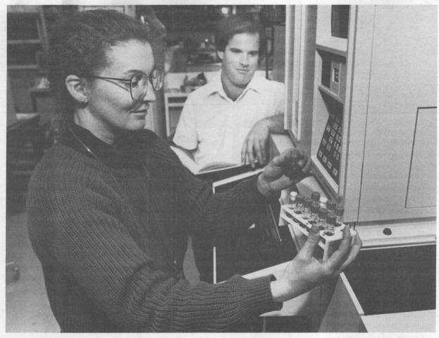
RACK OF NANOCLUSTERS — Sharon Craft (contractor) holds a rack containing solutions of nanoclusters, as she prepares to put a sample into a spectrometer for analysis. Jess Wilcoxon (1153) looks on. Some of the significant recent progress in the study of the small aggregates of atoms called nanoclusters has been made at Sandia.
